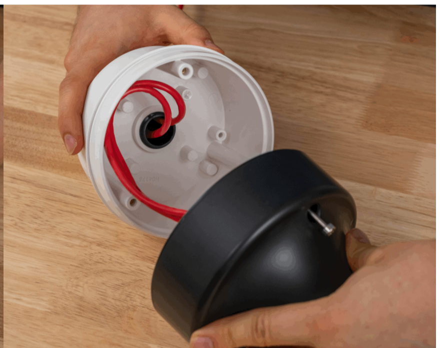
View of service loop
