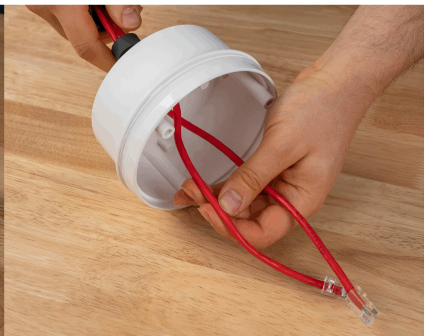
View of cable for service loop
