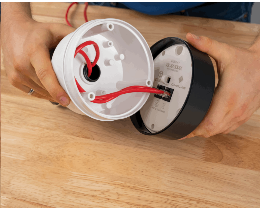
View of service loop
