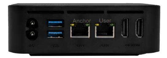
On the back of the mini PC, the Ethernet ports have been labeled with Anchor and User. The Anchor port is intended to connect to the Anchor Array and is configured for link-local addressing. The User port is intended to connect to the user's LAN using DHCP.
