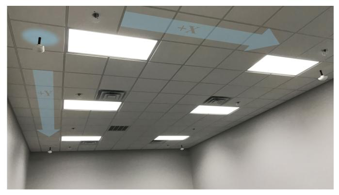
Note: the above images show the Anchors installed in a ceiling grid. It is recommended that users unfamiliar with system operation place Anchors on a tri-pod in an open area to gain familiarity with the system before doing a more permanent installation.
